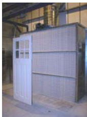
Caption: Hi-Tec Spray's high efficiency spray booth with heavy duty, manual conveyor track in operation at The Door Gallery.
